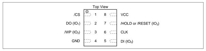
Figure 2b. 8-pad USON4x4 / WSON 5x6-mm (Package Code W)
