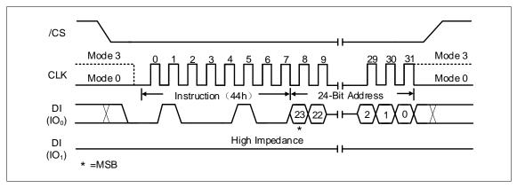
Figure 35. Erase Security Registers Instruction (SPI Mode only)
