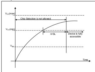
Figure 45a. Power-up Timing and Voltage Levels
