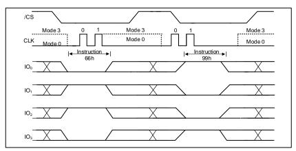
Figure 42b. Enable Reset and Reset Instruction Sequence (QPI Mode)
