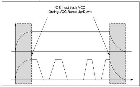
Figure 45b. Power-up, Power-Down Requirement
