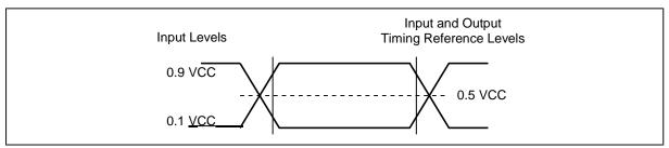
Figure 46. AC Measurement I/O Waveform
