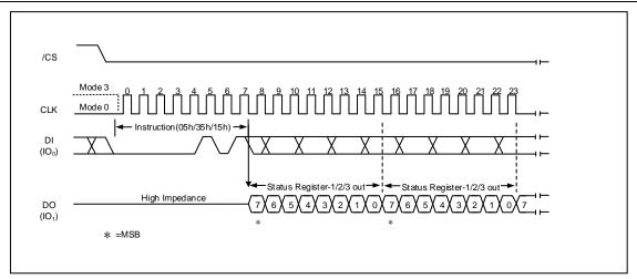
Figure 8a. Read Status Register Instruction (SPI Mode)
