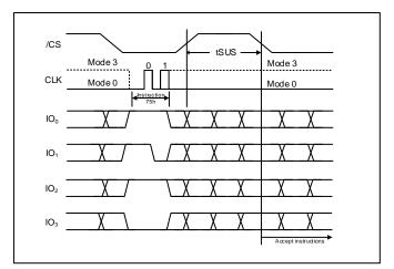
Figure 25b. Erase/Program Suspend Instruction (QPI Mode)
