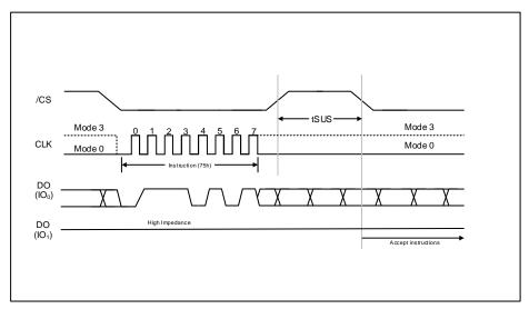
Figure 25a. Erase/Program Suspend Instruction (SPI Mode)
