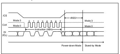
Figure 28a. Release Power-down Instruction (SPI Mode)
