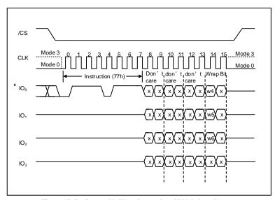
Figure 17. Set Burst with Wrap Instruction (SPI Mode only)
