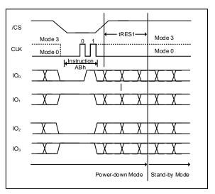
Figure 28b. Release Power-down Instruction (QPI Mode)
