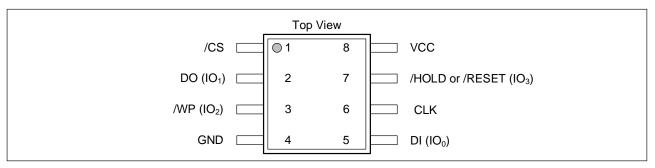
Figure 2a. 8-pin SOP / VSOP 208-mil (Package Code H, R)
