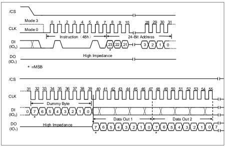
Figure 37. Read Security Registers Instruction (SPI Mode only)
